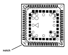
The math coprocessor also has a notch in one corner, marked by a dot, as shown below.
